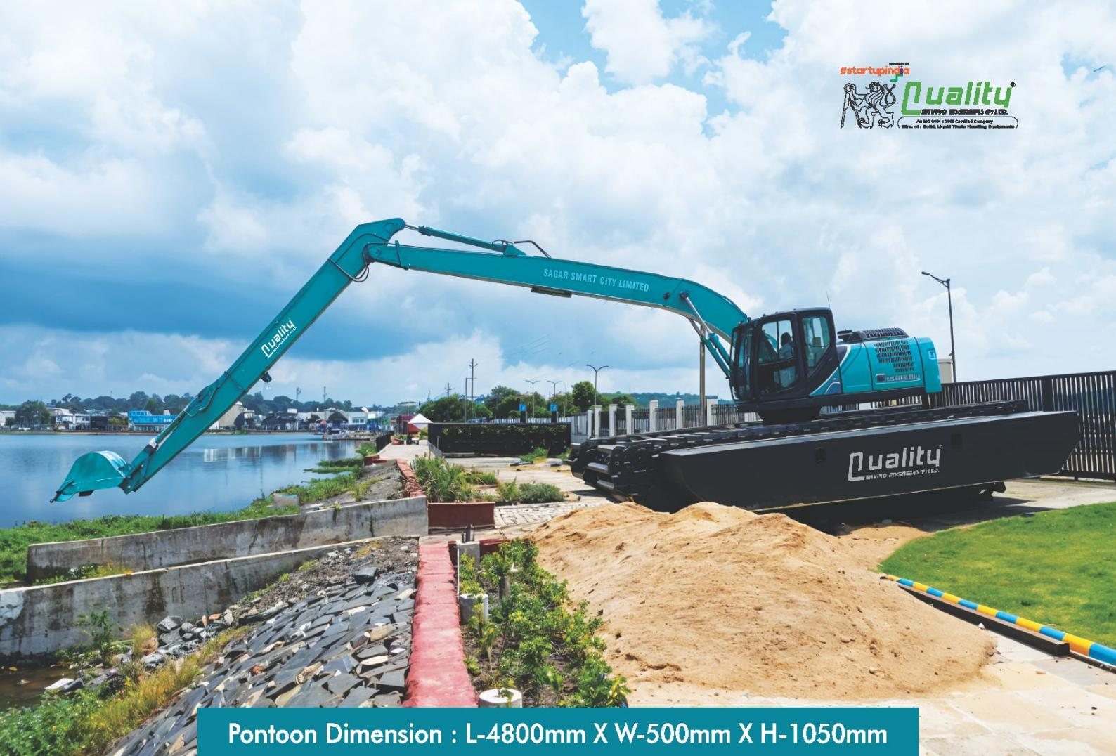
Pontoon Dimension : L-4800mm X W-500mm X H-1050mm
