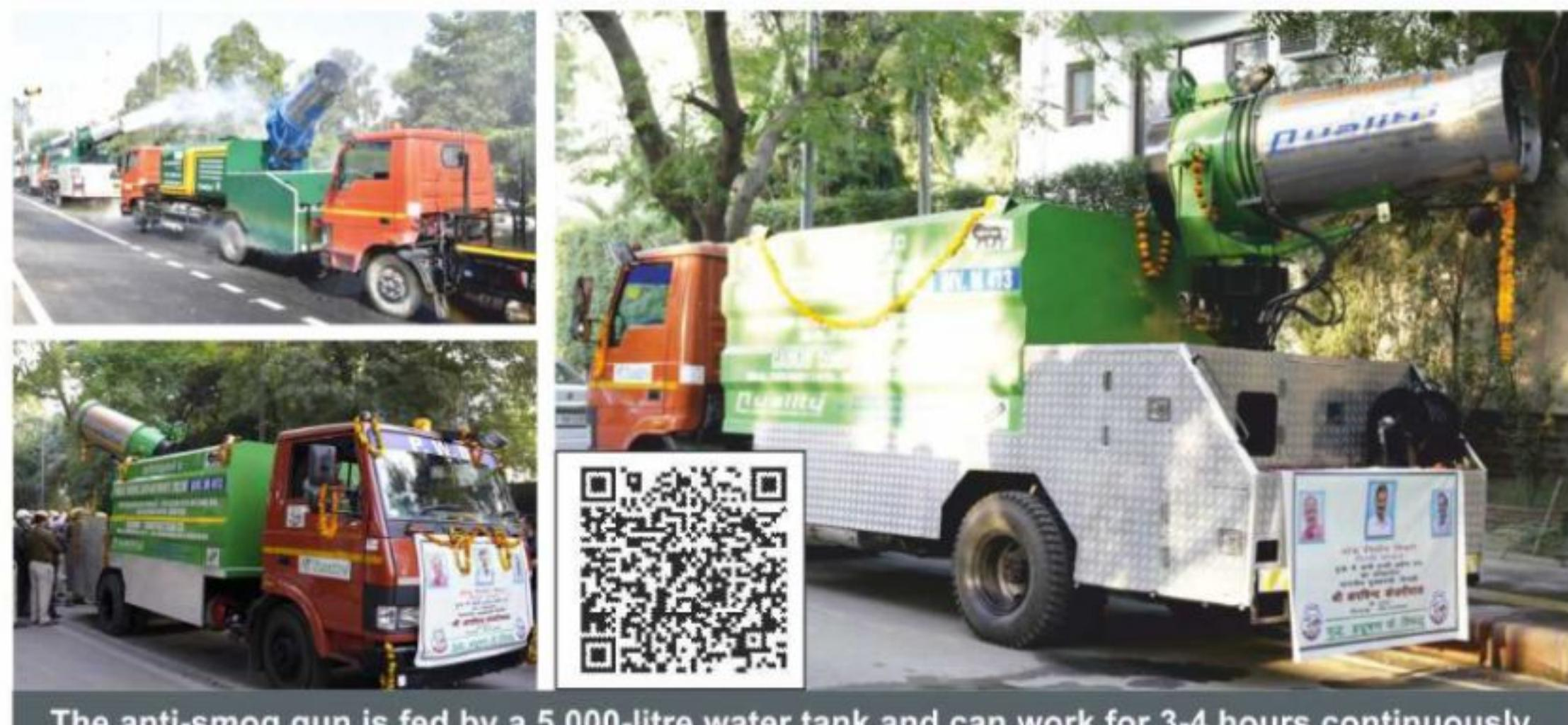
The anti-smog gun is fed by a 5,000-litre water tank and can work for 3-4 hours continuously.
